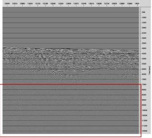
Fig. 8. The stacked section of 2D marine seismic data at CDP numbers 12800 to 14030 from multiple removals by the combination of SRME and parabolic Radon filtering, respectively.
