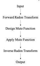
Fig. 4. The procedure of parabolic Radon filtering.
