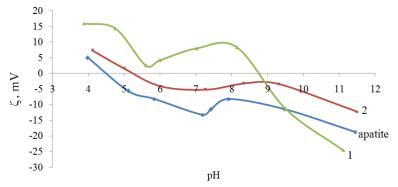
**Fig. 4.** The impact  $Fe^{3+}$  ions (1) and  $Ca^{2+}$  (2) ions on zeta potential of apatite:  $Ca^{2+}$  - 40 mg/l,  $Fe^{3+}$  - 40 mg/l
