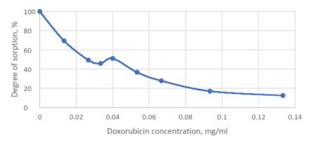
Fig. 6. Dependence of the degree of sorption of doxorubicin into chitosan-pectin microparticles (synthesized using a 20 mM CaCl<sub>2</sub> solution) on its concentration in suspension
