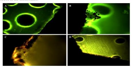
**Fig. 2.** Chitosan membranes in 1 % lactic acid solution under the epifluorescence microscope (x200), **A** –CS (1 %) membrane, **B** –CS (1 %) membrane with Lythri herba extract (0.5 g/L), **C** – CS (1 %) membrane with Lythri herba extract (1 g/L), **D** –CS (1 %) membrane with Lythri herba extract (2 g/L)
