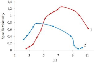
Fig. 5. The dependence of the specific viscosity of various solutions of flocculants depending on pH (1 - anionic flocculant, 2 - cationic flocculant)
