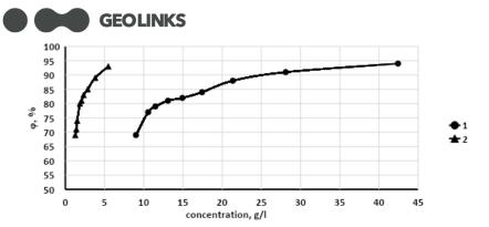
Fig. 3. Dependence of differential selectivity of the membrane UPM-100 on DNA (1) and nucleic acids (2) on the concentration of nucleic acids and DNA in the concentrate.
