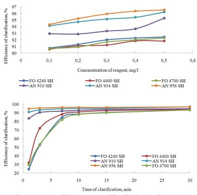
Fig. 6. Concentration and kinetic curves of the clarification degree of a model suspension of apatite concentrate in recycled water for a number of cationic (FO series) and anionic (AN series) flocculants
