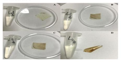
Fig. 4. CS membranes in 1% lactic acid tested. A - L1 (CS in 1 % lactic acid), B - L2 (mixture of CS 1 % in lactic acid + Lythri herba extract 0.5 g/L), C - L3 (mixture of CS 1 % in lactic acid + Lythri herba extract 1 g/L), D - L4 (mixture of 1 % CS in lactic acid + Lythri herba extract 2 g/L)
