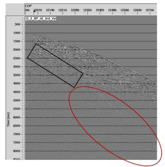
Fig. 7. The stacked section of 2D marine seismic data at CDP numbers 12000 to 12730 from multiple removals by the combination of SRME and parabolic Radon filtering, respectively.
