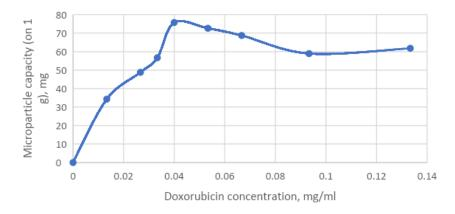
Fig. 7. Dependence of the amount of doxorubicin included in chitosan-pectin microparticles (synthesized using a 20 mM CaCl<sub>2</sub> solution) on its concentration in suspension
